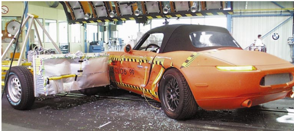
Bild 14: EU-Seitencrash Figure 14: EU side impact crash
