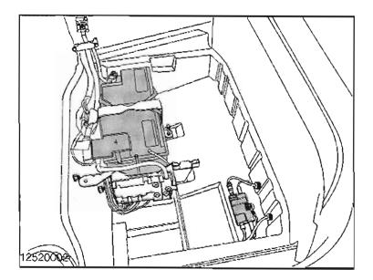
The glove box mounted fuse panel is located behind an access panel cover in the glovebox.
