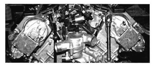
The S62 uses a high pressure (100 Bar) control system that ensures quick and reliable adjustments of the camshafts to meet the high performance requirements of the M Engines. The VANOS units are mounted directly on the front of the cylinder heads.
