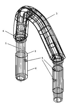
The rollbar is connected to the body mount by a sleeve.
