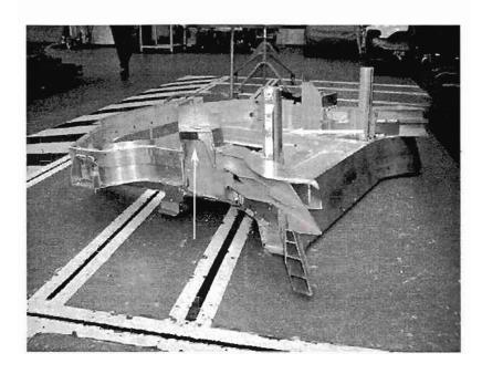
The left rear frame structure shown on the right highlights the upswept rear frame rail and the mounting point for the rear impact absorber.
