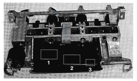
The IHKS control module is located on the back of the control panel.
