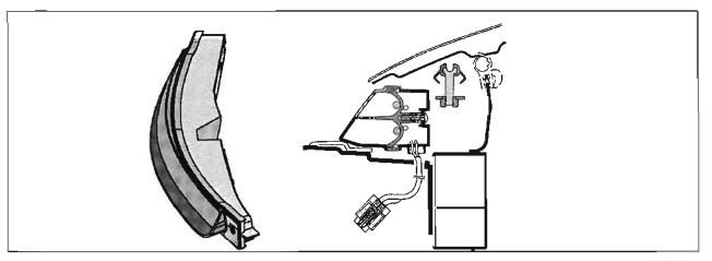
The neon lights are activated directly by the LCM. The neon tubes have ignition control units on each housing.
