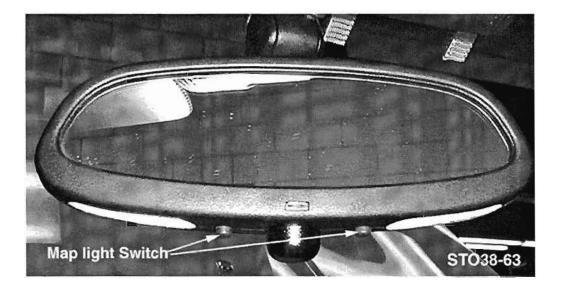
The switch provides a momentary ground signal that the GM recognizes as a request to either turn the lights on (if off) or turn the lights off (if on).
