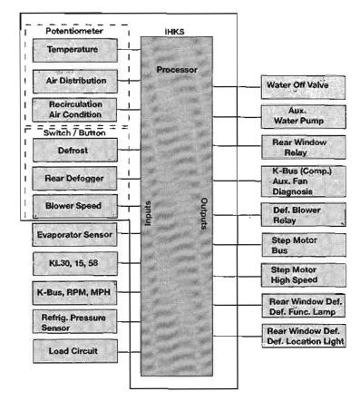
Note: If the IHKS control module is replaced, it must be recoded.
