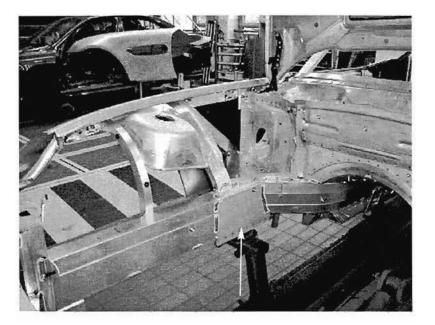
The left rear floor section shown here reveals the inner frame rail mounting to the rear support beam.
