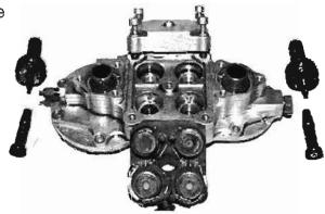
Two solenoids are required for each adjusting piston circuit, one for advancing and one for retarding the camshaft timing. The solenoids are controlled by the ECM.
