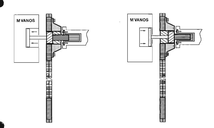
VANOS mechanical operation is dependent on oil pressure applied to position the control pistons. The double VANOS camshafts are infinitely adjustable within the mechanical travel limits of the drive gears.
