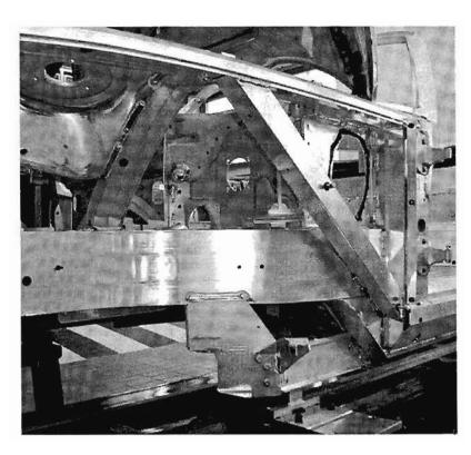
The front structure illustration on the right highlights the additional frame support behind the front bumper assembly.
