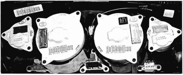
• The instrument cluster assembly is hard wired to the IKE module which is located behind the glove box.
