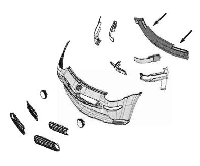
Pull out (unsnap) the grille panel to access the tow hook mount-ing point.
