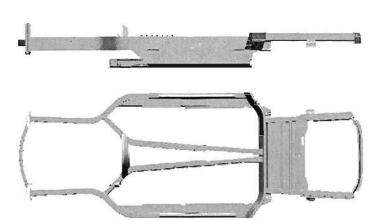
The frame and floor pan assembly illustration on the right shows additional triangulation reinforcement pieces.
