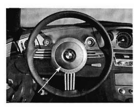
To remove the airbag - compress the spring latches through the two access holes (at the bag base, next to the steering wheel spokes).
