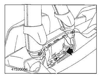
The roll bar has been removed from the mounting sleeves to allow visibility of the single mounting bolt on the right, and the four bolt locating plate on the left.
