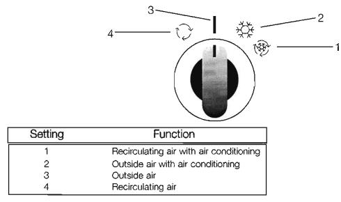
The recirculation air control flap is operated by a stepper motor (bus).
