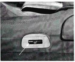
The two position Seat Heater Switches are located on the left and right sides of the center console as shown above.
