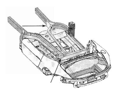
Shown on the right is the windshield frame structural mounting and engine compartment bulkhead assembly.
