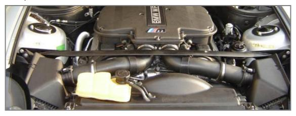
In our oppinion the instalation of the Performance Package can provide increased protection to the strut towers and in extreme cases the frame as well, especially in unforeseen situations, (e.g. sliding on wet pavement and subsequently hitting the curb violently).
