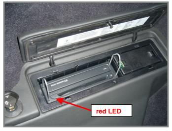
Attention: before the GPS unit is removed the ignition has to be turned off and all other electrical instrumentations need to be off as well. The red LED on the GPS unit (see arrow) must not be blinking anymore! This will occur automatically a few minutes after the ignition has been turned off.
