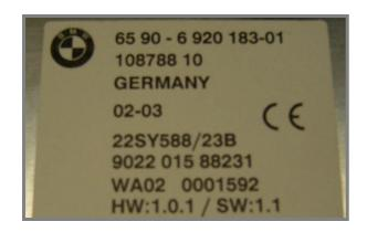
ID sticker of the original GPS unit of a BMW Z8 Bj. 04/2003. On the replacement unit the correct part number is printed on the first line: 65 90 - 6 942 911.
